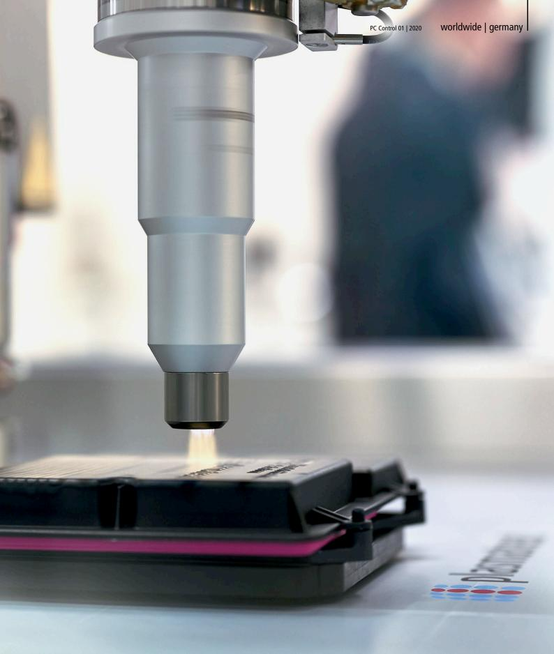
No need to move the plasma jet: A floating planar mover carries the workpiece exactly into position for surface treatment.
