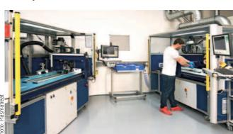
**Fig. 5:** Advanced restructuring: Plasma system and bonding station facing one another. The components can be bonded and further processed immediately after pretreatment.
