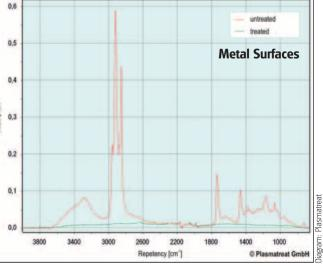
**Fig. 3:** Infrared spectroscopic measurement: During the microfine cleaning of metal surfaces, Openair-Plasma removes all impurities and organic contaminants such as grease, oils and water adhering to the boundary layer.
