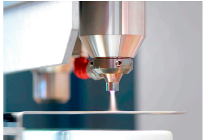
Fig. 1: The chemical-physical Plasma-SealTight process enables the area-selective deposition of functional nanocoatings in milliseconds and thus the creation of covalent bonds between different materials
