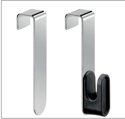
Fig. 3: The metal body (left) can be overmolded with the thermoplastic compound (right) immediately after atmospheric pressure plasma coating to produce a strong joint
