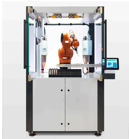
Fig. 10: The turnkey, fully automated PTU1212 plasma cell contains everything the plasma process needs and can be connected to any conventional injection molding machine
