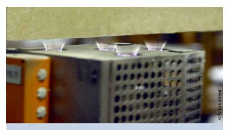
Due to activation by plasma the plastic-coated sheet steel covering layers of the sandwich panels are given new surface properties amenable to adhesion.
