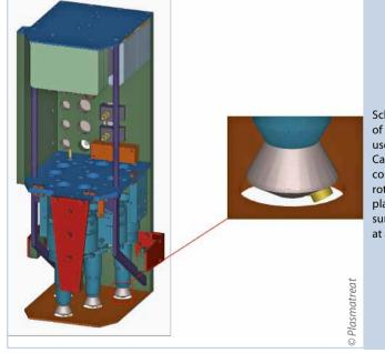
Schematic illustration of plasma generator used at Schmitz Cargobull's containing four rotary jets. The plasma strikes the surface to be treated at an angle of 45°.
