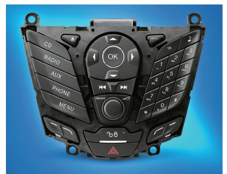
Fig. 5: The integrated control panel (ICP) forms the centrepiece of the dashboard; the plastic switches are pretreated with atmospheric plasma before painting to ensure a flawless finish and an adhesion that will last for years (Photo Plasmatrete)
