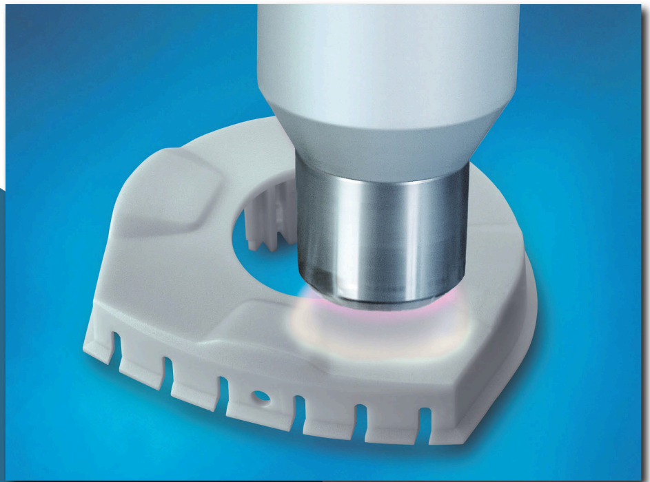
High effective surface activation by atmospheric plasma treatment (Photo: Plasmatreat GmbH)
