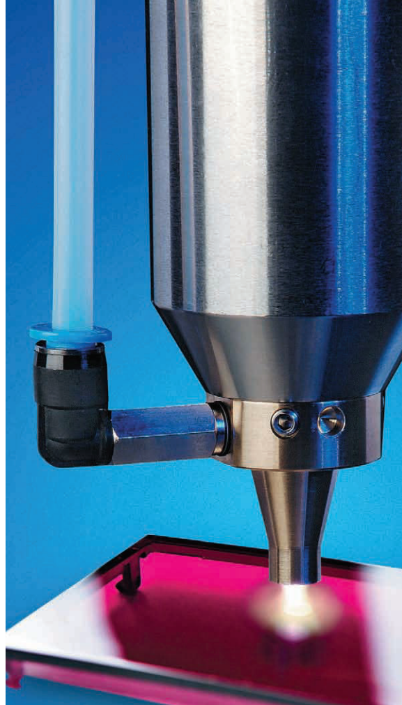
Fig. 1: Locally selective plasma coating under atmospheric pressure: the chemical composition can be varied according to the application to obtain the best results for a variety of different materials. Photo: Plasmatrete
