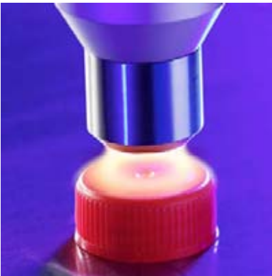
Fig. 4 Abrasion-resistant imprints are required especially in the food industry. The plasma ensures optimum adhesion properties (Photo: Plasmatreat)
