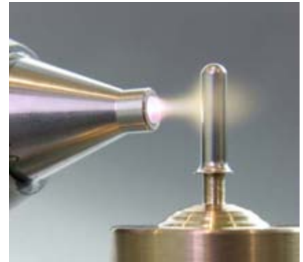
Fig. 7 Brilliant surfaces are achieved in automotive engineering by pretreatment with atmospheric-pressure plasma prior to painting (Photo: Plasmatreat).
