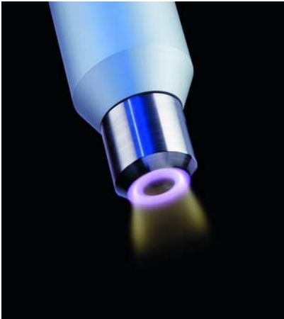
Fig.1: The new 49 m long coil coating plant at Griesser AG by dispensing with a cleaning line establishes a milestone in process engineering. Fig.2: The electrically neutral plasma beam allows ultrafine cleaning, high activation and extremely thin coating of surfaces. Fig.3: By realizing his vision of environmentally friendly precleaning in the coil coating process project leader Branko Vasiljevic achieved a worldwide success. (Photo: Blue Rondo International)
