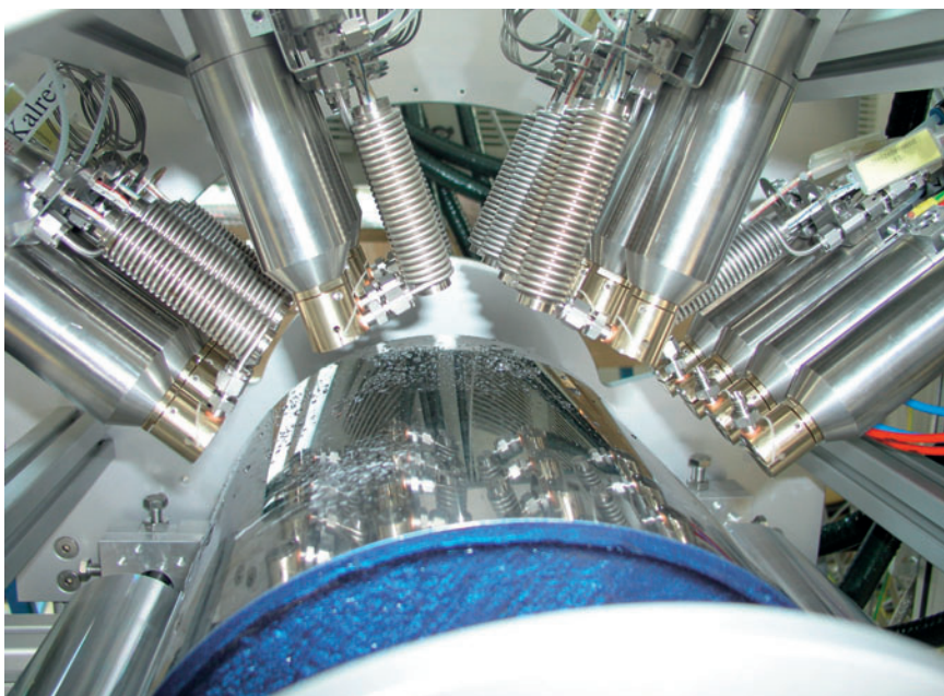
Fig. 7. Flexible nozzle system with specially developed evaporation, in which the gap between the nozzles can be adjusted at will
