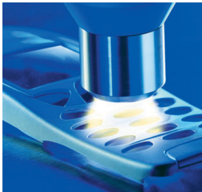
Fig. 5. Following pretreatment with Openair plasma, display windows made of polycarbonate can be bonded into the half-shells of mobile phone housings with solvent-free UV adhesives
